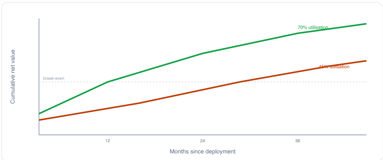
Figure 6.2 — Modeled payback curves. Utilisation, not robot count, determines when a fleet crosses break-even.
